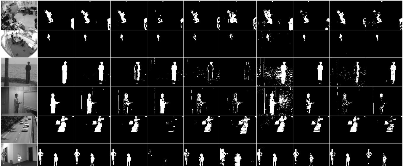
Fig. 9. Comparison results on different sequences. First to sixth rows: Detection results on 221th frame of Fighting , 216th frame of Intelligent room , 1615th frame of WaterSurface , 23857th frame of Meeting room , 1615th frame of Highway , and 338th frame of Dance bootstrapping sequences. First and second columns: Original image and its ground truth. Third to eleventh columns: Results of JVFS-D-RPCA, RPCA, GoDec, RPCA-ME, PCA, MD, SOBS, GMM, and KDE, respectively.
